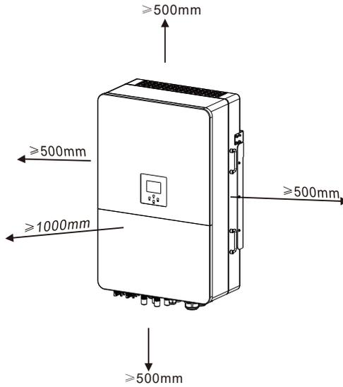
For a proper ventilation of the inverter and avoid overheating, allow a clearance of approximately 50 cm around the inverter and at least 100 cm to the front as it can be seen at the picture below.
