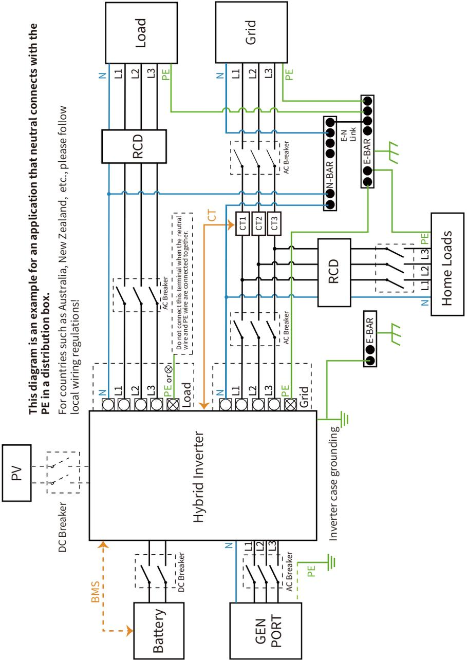
This diagram is an example for an application that neutral connects with the PE in a distribution box.
