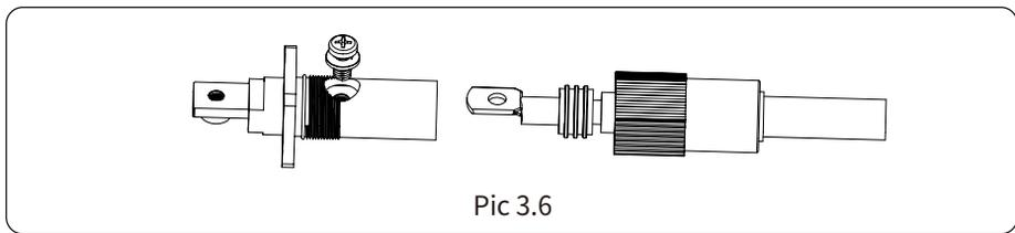
e) Fasten the terminal with outer cover, as shown in Pic 3.7.
