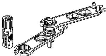
Pic 5.5 connector with cap nut screwed on
